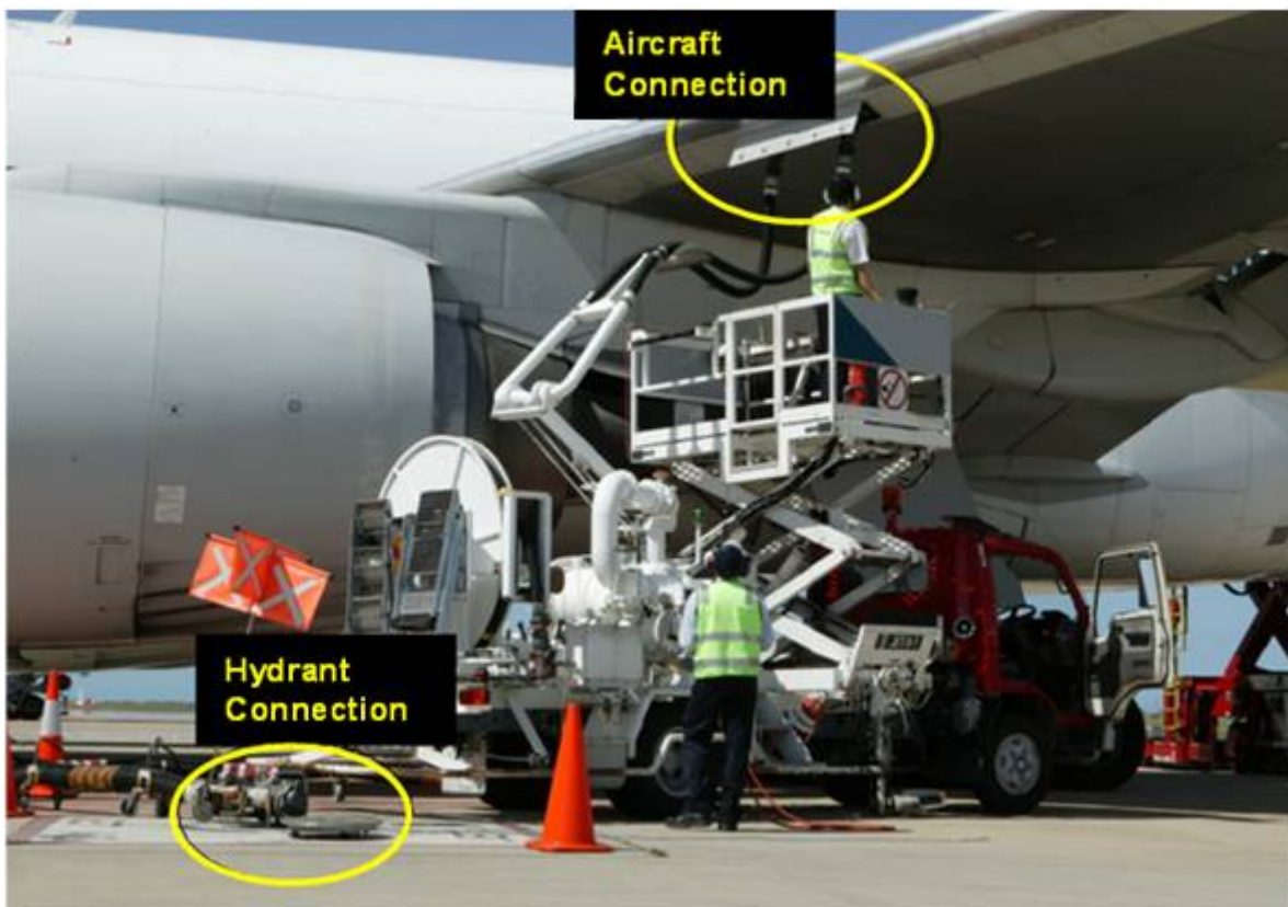
Figure 2 – Fueling 'underwing' via a hydrant connection
