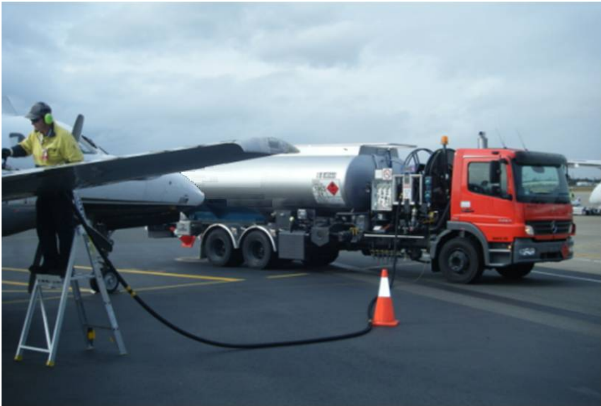
Figure 3 – Fuelling 'overwing' via a tanker
