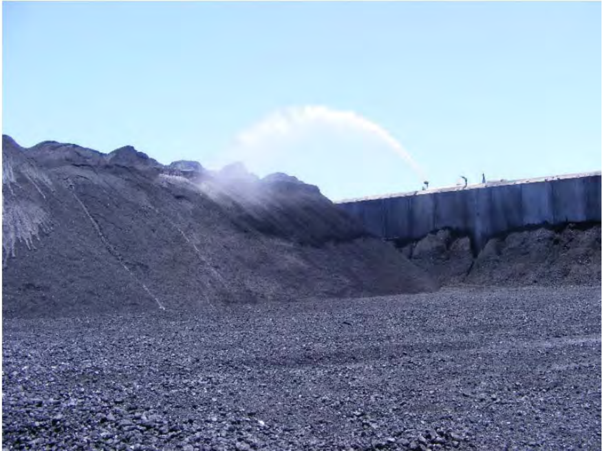
Stockpile application of veneering agent from bund way – DBCT P/L 2009
